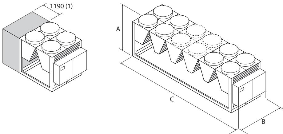
(1) Additional module needed to contain the hydronic kit with "accumulation" option in sizes:
