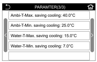
You can press on any parameter to alter its value. Every parameter modification page has an "OK" button for saving the values entered, and an "X" button (at the top right) if you don't want to save the value modifications; if one of these two buttons is pressed, you will quit the setting page and return to the parameter selection page:
