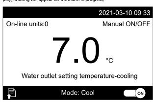
NB: if the user does not carry out any operations on the display for 10 minutes the screen will automatically return to the homepage, except where the system sends notifications that require the user to push the "Ok" or "Cancel" buttons, for example, notification that the defrosting cycle has been completed, shown in the following image;
