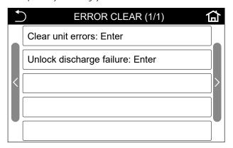
Press the "Clear unit errors" button to access the page for deleting the errors that have arisen on the unit:
