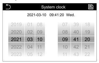
Date and time will be displayed in the following format: YYYY - MM - DD / HH:MM:SS The date and time can be selected by scrolling the rollers until the desired data is obtained; pressing the top right icon will save the data, while pressing the top left icon will clear the page; both will return the display to the top level;
