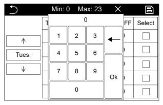
Once a time band has been set, press the corresponding empty box in the "Select" column; a tick will appear, indicating that the time band has been activated; To save the set data, press the icon in the upper right-hand corner ( , while if you wish to exit without saving, press the one in the top left-hand corner ( );
