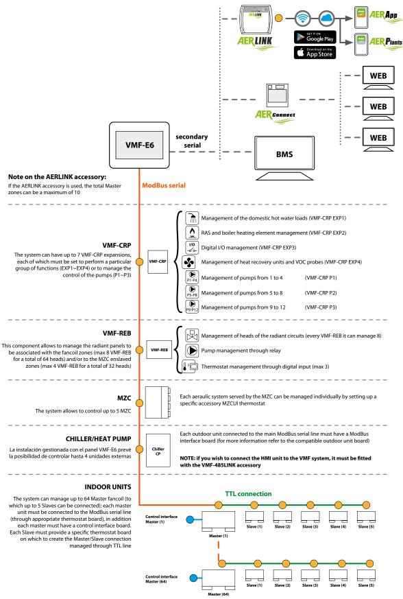
**ATTENTION:** if one (or more) areas are controlled with an FCWI fan coil (each of which require the VMF-485LINK interface), these areas cannot have a Slave unit
