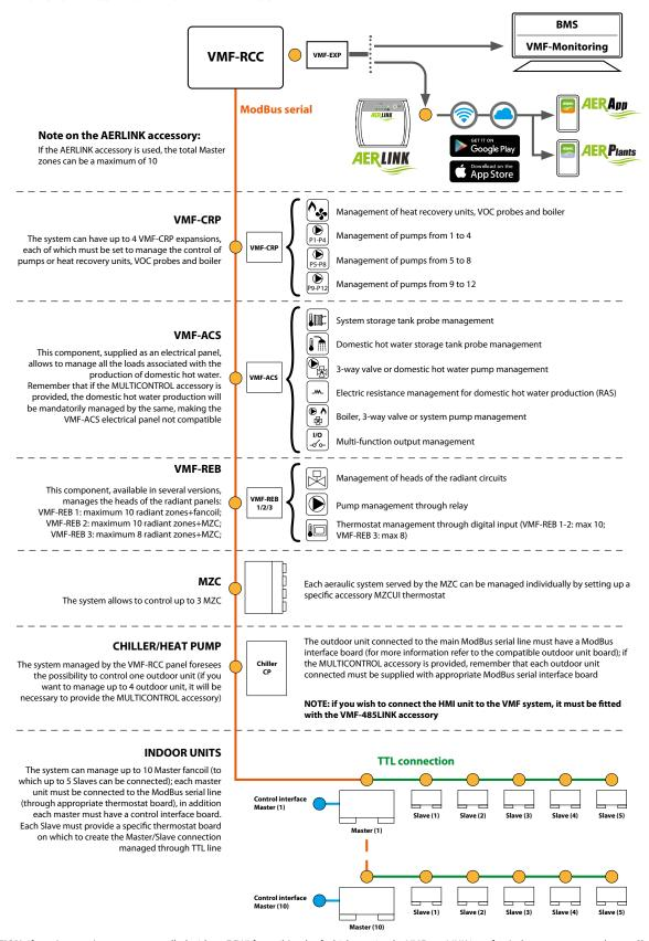
**ATTENTION:** if one (or more) areas are controlled with an FCWI fan coil (each of which require the VMF-485LINK interface), these areas cannot have a Slave unit.
