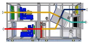
In night time mode the unit modifies the operating settings to adapt to the changes of evaporation from the pool and reduce consumption to the minimum.
